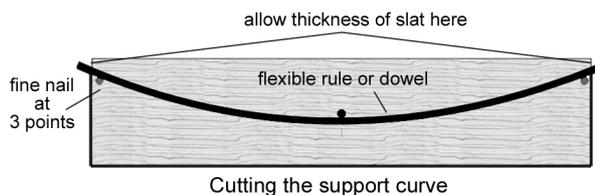
The curve can be as gentle or steep as you like, but make sure that you leave enough "meat" to provide adequate support ... a minimum of 45mm is suggested if you are using 100mm x 25mm (nominal) timber. Drive in a fine nail at each of the points and using a flexible ruler or piece of fine dowel, bend it around the nails and then draw your curve using the ruler or dowel as a guide.
