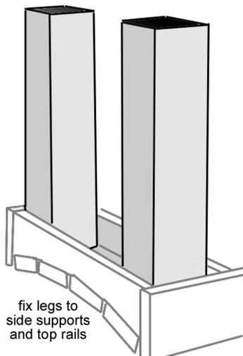
Measure up equally from the bottom of each leg and fix the bottom rails to the legs. Fix the short ends first by lining them up with the edges of the legs and then fix the two long sides.
